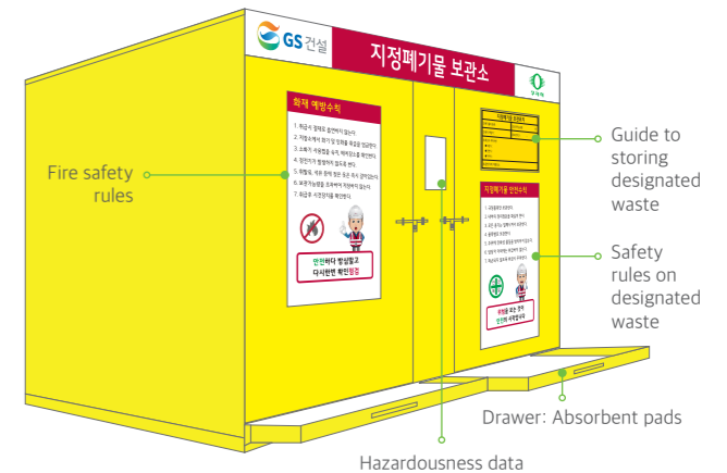
Designated waste storage installation specification
