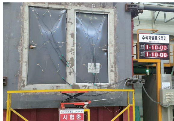
Fire resistance test of fire doors
